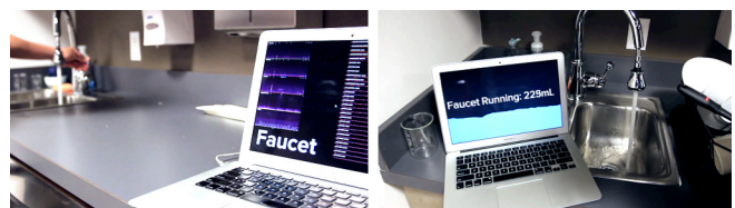
Figure 17. A first-order “faucet running” synthetic sensor (left) can be used to power a second-order “water volume” synthetic sensor (right).
