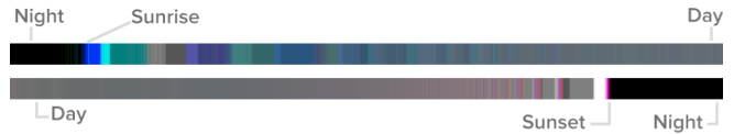
Figure 10: Light color captured over a one-hour period from an example sunrise (top) and sunset (bottom).
