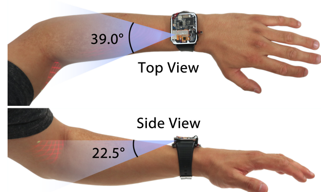
Figure 3. Top and side view of LumiWatch, with illustration of projector’s field of view. Top: tangential field of view. Bottom: axial field of view.
