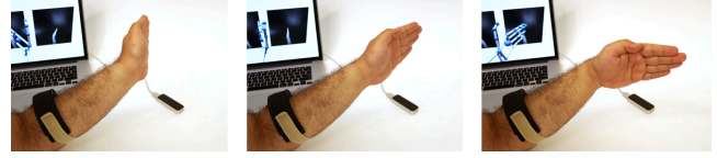
Figure 17. Our wrist angle task used a Leap Motion controller to provide ground truth. Participants swept their wrist from left to right (with all intermediate angles recorded).
