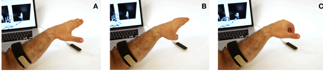
Figure 19. Our coarse hand pose task evaluated tracking of the thumb (A \rightarrow B) and four other fingers (A \rightarrow C). We used a Leap Motion controller for ground truth.
