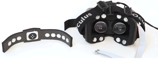
Figure 21. Interferi could be integrated into future smartwatch wristbands and AR/VR headset liners, as seen in these hardware mock-ups.
