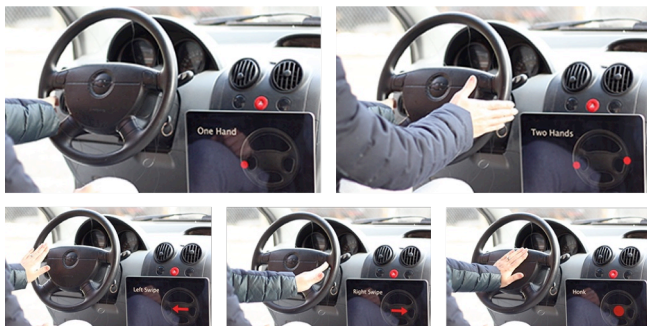
Figure 20. This Electrick-augmented steering wheel can track hand location and gestures.
