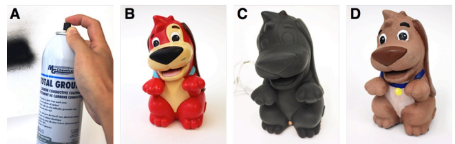
Figure 5. We carbon sprayed (A) an off-the-shelf toy (B) to make it interactive. A new topcoat was applied (C to D).
