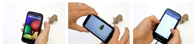
Figure 21. This Electrick-augmented phone enclosure allows different grips to launch apps.
